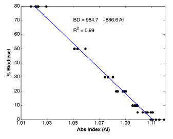
Figure 5. Transformed relation between blend level and absorbance index; dilution 1:2915.
