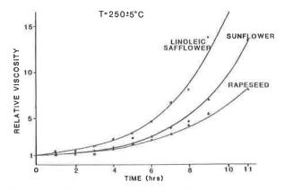
FIG. 2. Oxidative polymerization rates of three vegetable oils,
