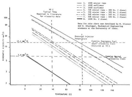
FIG. 3. Viscosity vs temperature for vegetable oil blends.
